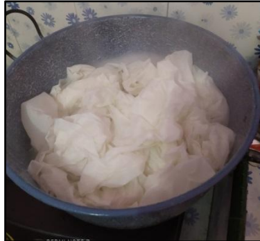
Figure 3 Process of Boiling Primisima Cotton Fabric with Mordan Material
